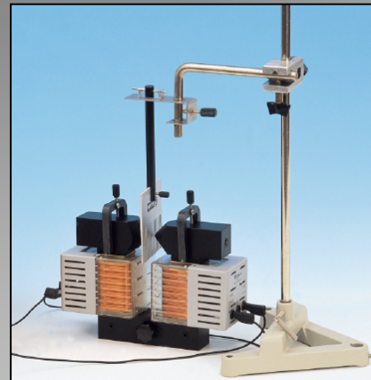
Waltenhofen's pendulum : demonstration of an eddy-current brake
